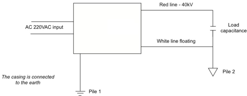
Wiring description: The grounding bolt of the rear panel of the product is grounded by the pile 1. The black terminal of the rear panel is connected to the floating white line, and the capacitor is negative, that is, the ground pile 2 in the above figure.
