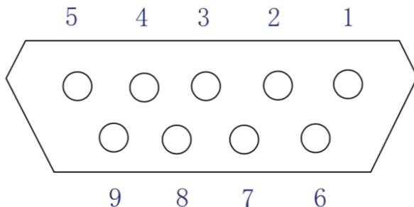
**\*\*DB9 control pin description The port on the power supply board is the female connector. It needs to be equipped with a male connector to complete the corresponding control function.\*\***
